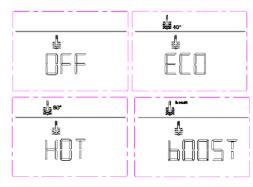
This icon will flash until the predetermined water temperature is reached.
