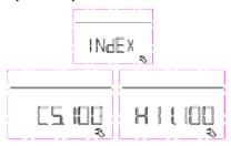
C5.1000-- LCD switch version H11.100-- master controller version
