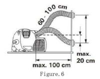
After the intake and exhaust pipes are inserted through the through holes, if it is necessary to shorten a section, the exhaust pipe shall be slightly shorter than the intake pipe. Avoid excessive expansion or tension on the exhaust pipe.
