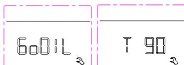
Click on the rotary button to enter the fast pump oil. The default fast pump time is 90 seconds. The remaining time can be adjusted with a knob.
