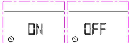
The time switch is only enabled once until it is disabled (turned off) or powered down. If the time switch is programmed and enabled, the time switch icon is displayed in the status line (2). The timing icon flashes if the time switch is enabled and activated.
