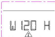
A manually recovered fault means that the fault code is displayed in the parameter setting field (7) when the fault occurs. The cause of the fault can be determined and remedied by the help of the troubleshooting guide. The fault code disappears after a few seconds, and the warning disappears, and the warning symbol is displayed in the menu bar (4).
