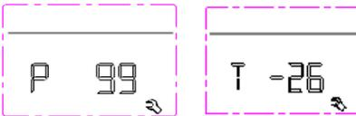
Use the rotary button to switch between atmospheric pressure and ambient temperature.
